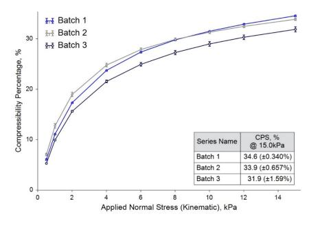
Batch 3 exhibited a lower Compressibility than the other two samples. Low Compressibility indicates that a powder is more uniformly packed and entrains less air within the bulk. This is a property typically associated with more free-flowing powders.
