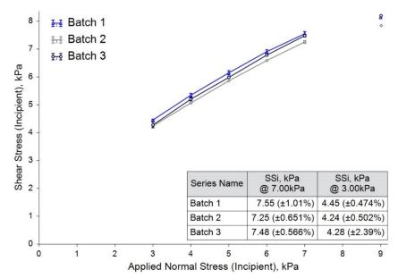
Limited differentiation was observed between the three samples in this test. Furthermore, the yield loci for the samples are not linear, meaning that Mohr's circle analysis of the data, which relies on the application of a Best Fit Line to the data, will not generate parameters that accurately describe the behaviour of the powder.
