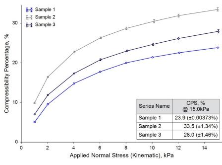
Sample 2 was more compressible than Sample 1, indicating that it entrained a greater proportion of air within its bulk, which is typical of more cohesive powders. High Compressibility can contribute to poor behaviour in operations where a powder is subjected to an applied force, for example as a consequence of storage in large quantities.
