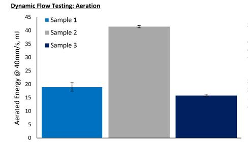
Sample 2 generated a considerably higher Aerated Energy (AE) than Sample 1, indicating greater cohesive strength between the particles. High AE can contribute to poor flowability in situations where uniform aeration of the powder is necessary, such as the aerated conveyor.
