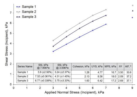
Sample 2 generated higher Shear Stress and Cohesion values and a lower Flow Function than Sample 1, indicating that it is likely to be more problematic when required to flow under high stress, low flow conditions such as in large hoppers.
