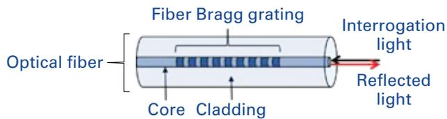
gratings (FBGs). An FBG, shown in Figure 2, is a short segment or structure of varying refractive index within the core of an optical fiber; cladding surrounds the FBG to give it mechanical integrity. A critical characteristic of an FBG is that the application of flow force induces a shift in the wavelength of interrogation light that it reflects.
