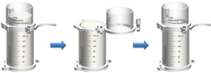
Figure 15: Vessel splitting is an effective way of generating a precisely known powder volume and a level surface, for the accurate determination of bulk density.
