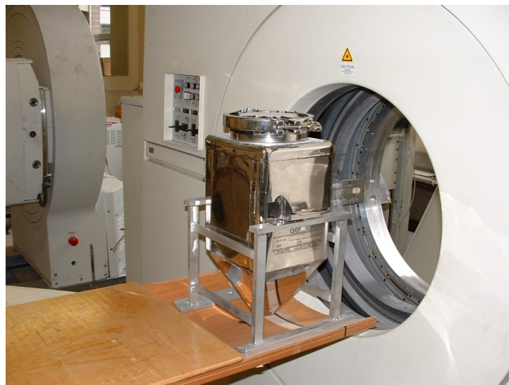
Figure 1: A mixing vessel entering the PET camera to enable measurement of the extent of homogeneity within the blend
